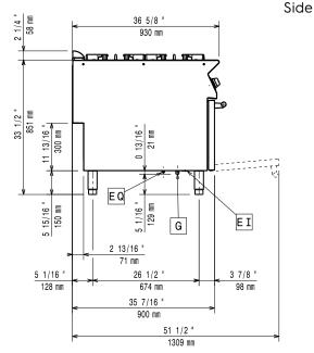
Electrical inlet (power) Gas connection
