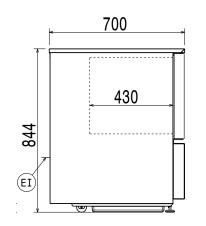
EI = Electrical inlet (power) RO = Refrigerant Outlet
