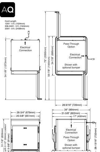
\*33-3/8" (848mm) - with optional 3-1/2" (89mm) casters \*35-1/4" (894mm) - with optional 5" (127mm) casters \*33-3/4" (857mm) - with optional 6" (152mm) legs
