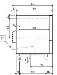
D = Drain El = Electrical inlet (power)
